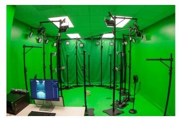
In Providence's UPmersiv\* Studio, an Intel-powered Evercoast workstation equipped with Intel® Xeon® processors is connected to 20 RGB-D cameras. The depth-sensing cameras provide the ability to only accept video from within the capture ring, which is about seven and a half feet in diameter. Each camera captures a different angle of the actor.
