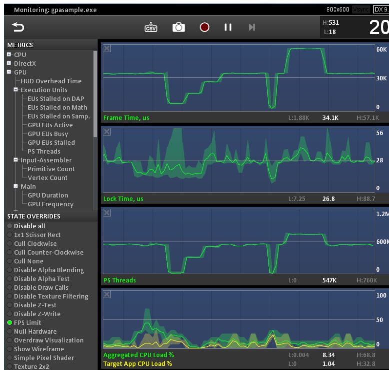
Figure 3-2: Or use the Intel® Graphics Performance Analyzers System Analyzer to show real-time stats
