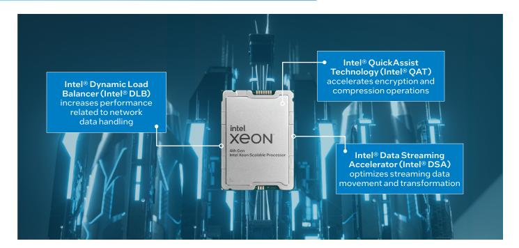
Hardware accelerators built into the processor dramatically improve performance by offloading tasks critical to CDN operation from the processor cores to dedicated hardware resources, which also frees up processor cores for other work. In addition to its throughput benefits, this approach improves latency and energy efficiency by avoiding data transfer to off-processor hardware through the PCIe bus.
