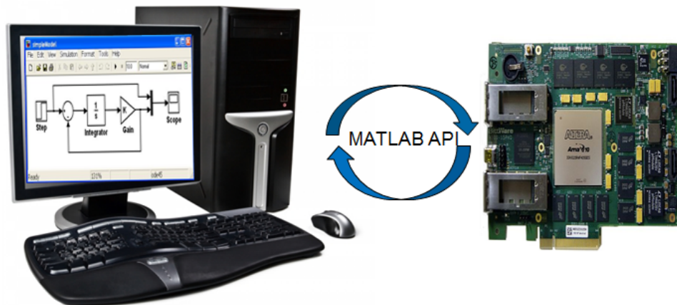
Figure 20. Hardware in the Loop Host-Target Setup
